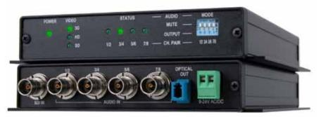
The Fiberlink® 3360 Series allows you to transmit 3G, HD or SD-SDI as per SMPTE 424M-2006, 292 and 259 with the ability to embed up to 8 channels (4 pairs) of AES/EBU digital audio. Convenient switches on the 3360 Series transmitter allow the operator to embed each of the four pairs of audio independently, to strip previously serialized audio, or to pass it through without modification. At the receive end of the fiber optic link, the operator can decide which audio pairs they need de-embedded.
